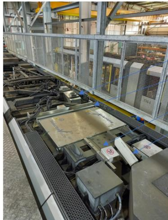
Figure 3 OLE measurement equipment installed on the roof of tram 3071
